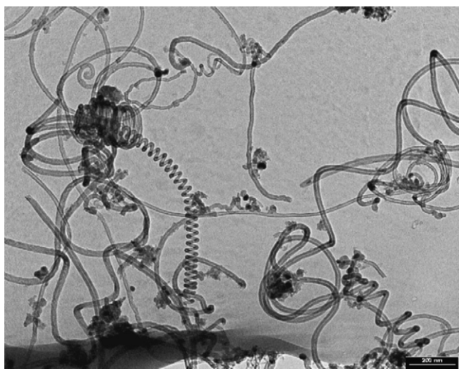
Fig. 6. CNTs on 2.5 wt% Co-2.5 wt% Pr/SiO 2 catalyst prepared by the IAP method.
